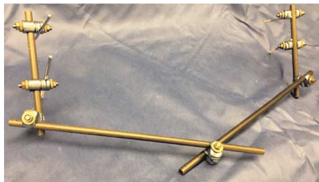
FIGURE 2. A pelvic frame with four adjustable clamps, two carbon fiber reinforced epoxy, four 316L stainless steel Schanz pins, two large combination clamps, and one tube-to-tube clamp.
