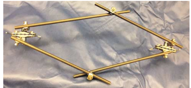
FIGURE 1. A diamond-shaped Synthes large external fixator with four stainless steel Schanz pins, four graphite rods, two combination clamps, two six position multi clamps, and two rod attachments similar to the construct studied by Luechinger et al. 13
