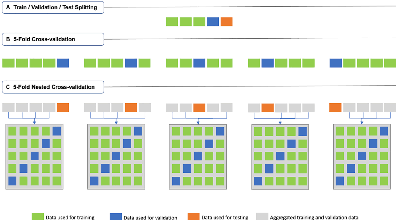
Figure 3: Schematic description of (A) traditional train-validation-test splitting, (B) fivefold cross-validation ( k = 5 ; where k is the number of folds), and (C) fivefold nested cross-validation ( k = m = 5 ; where k is the number of folds in the first-level cross-validation, and m is the number of folds in the second-level cross-validation).
