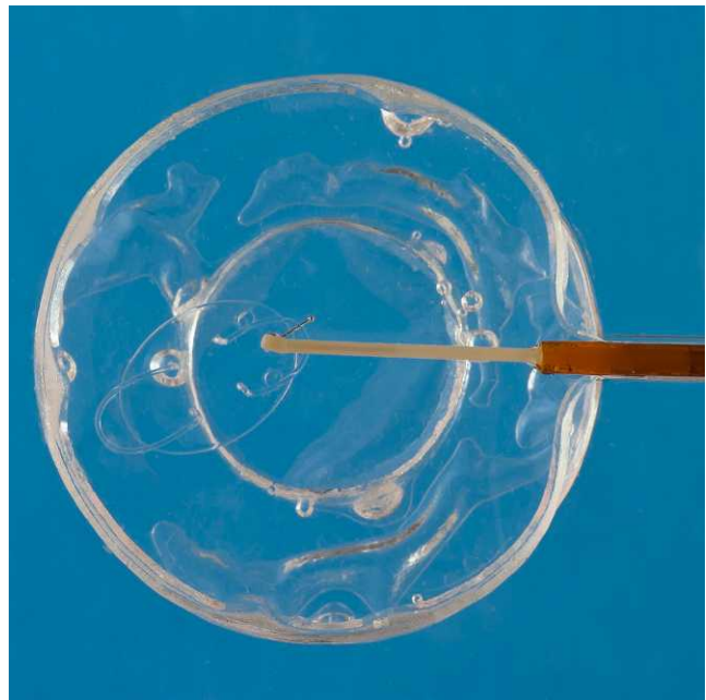
FIGURE 1. For evaluation of radio-frequency heating, IOLs were individually placed in a small chamber. A fiber-optic temperature sensor (Opsens) was positioned as close to the IOL as possible. Temperature was monitored during a multi-slice GRE sequence with high power settings.
