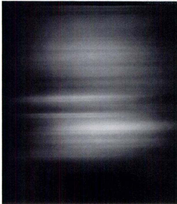
Figure 1 MR image with 2 phase encoding steps.
