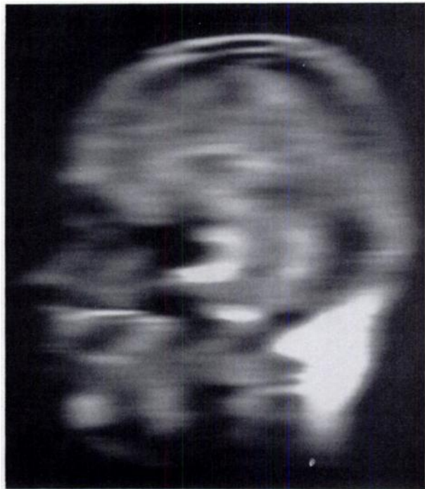
Figure 4 MR image with 12 phase encoding steps.
