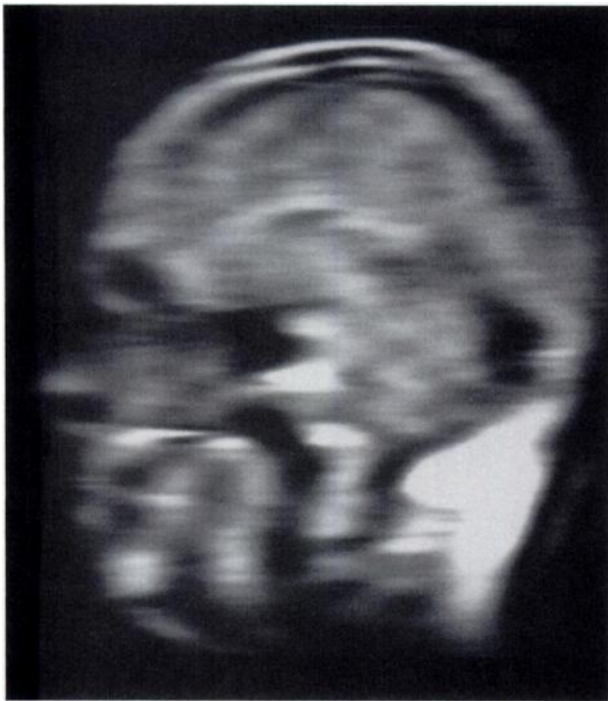
Figure 5 MR image with 16 phase encoding steps.
