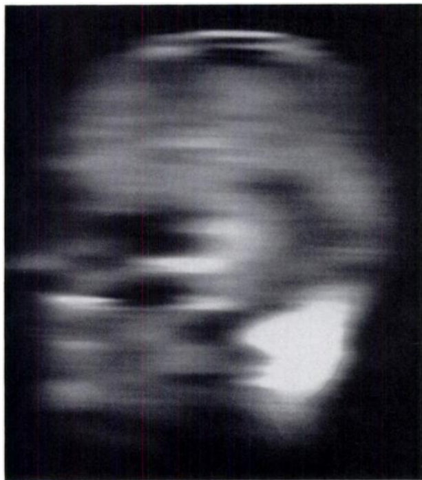
Figure 3 MR image with 8 phase encoding steps.
