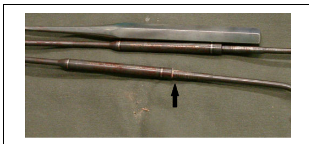
Figure 11. Calcified deposits at the extendable portion of the rod.
