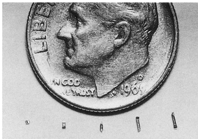
Figure 1. Examples of metallic (steel) foreign bodies used in experiment. The diameter of each is 0.39 mm. The lengths range from 0.4 to 1.5 mm. The corresponding volumes range from 0.048 to 0.179 mm 3 . A United States dime is shown for size comparison.
